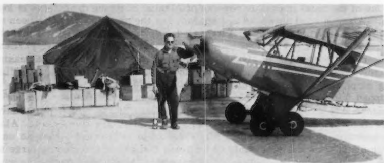
FIG. 5.—SMALL AIRPLANE USED TO SUPPORT SURVEY PARTIES. THIS ONE IS EQUIPPED WITH TANDEM WHEEL LANDING GEAR.
